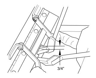
Figure 6-7 Gap Measurement
